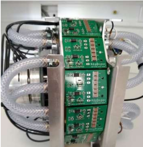
Axial flux electric machine with integrated power electronics
