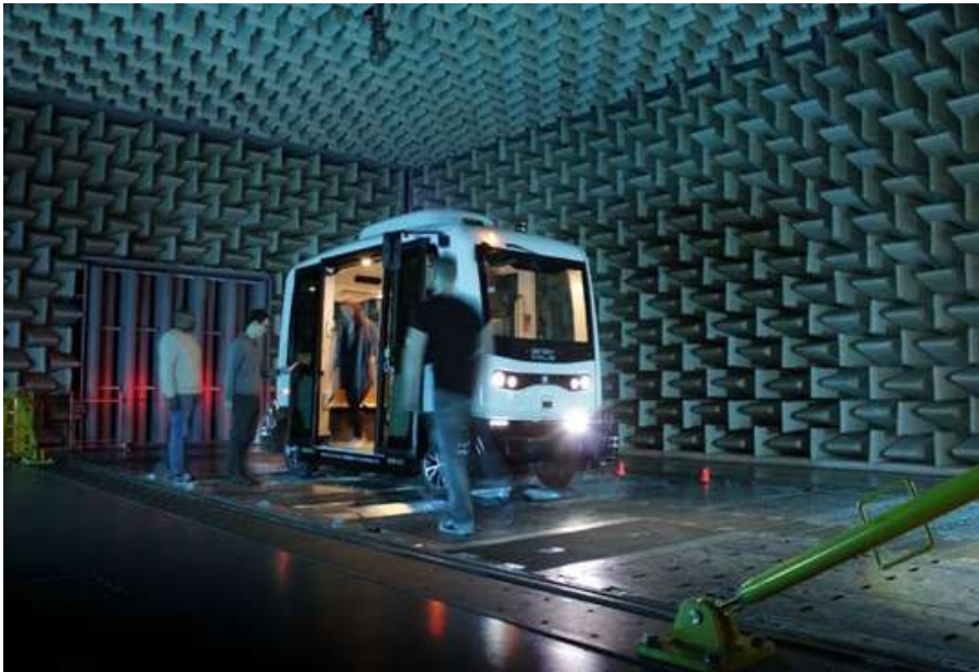
Autonomous shuttle in KIT's acoustic four-wheel roller dynamometer
