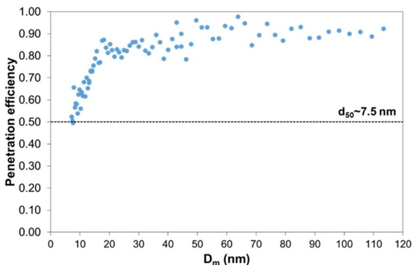
Figure 3. The solid particle penetration efficiency of the prototype Sampling & Conditioning Particle System (SCPS).
