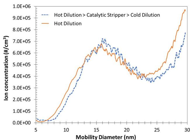
Figure 1. Sub-23nm engine particles size distribution measured with the HM-DMA in hot operation using a PMP-compliant setup and a single step hot dilution.
